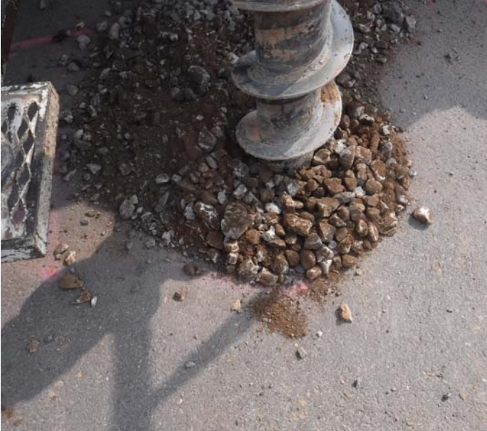
PHOTO NO. 29: General view of gravelly soils encountered in vertical boring B-6.
