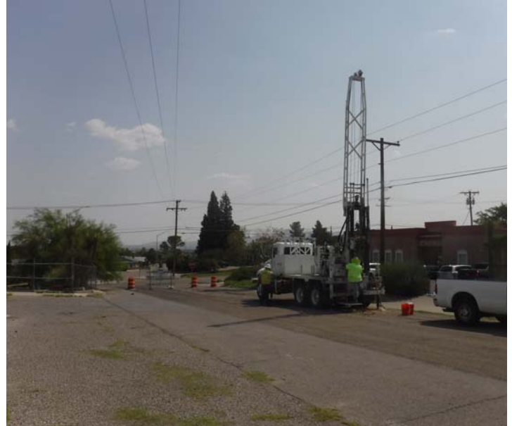
PHOTO NO. 26: General view of our subsurface soil drilling operations at vertical boring B-9.
