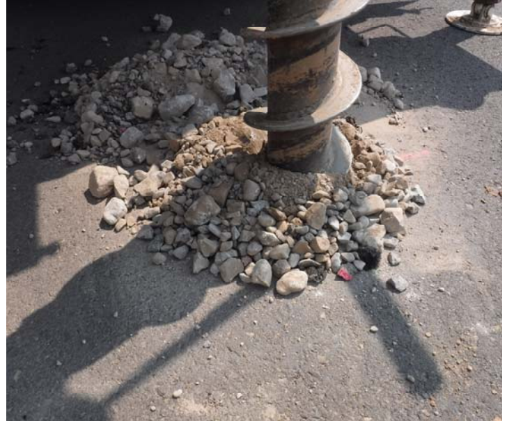
PHOTO NO. 30: General view of gravelly soils encountered in vertical boring B-7.
