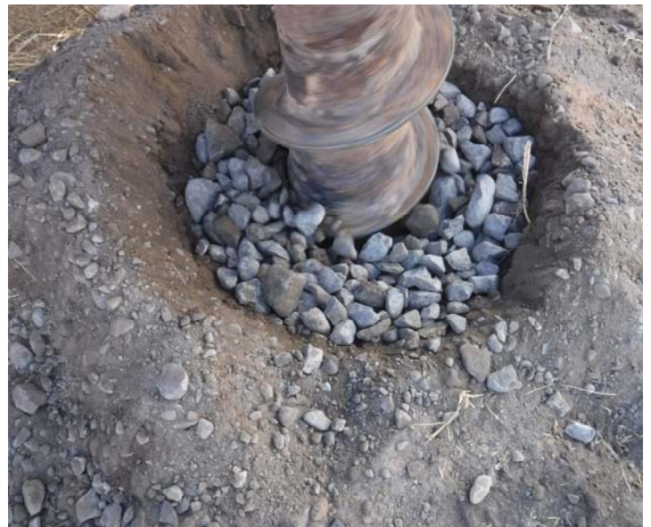
PHOTO NO. 48: General view of gravelly soils encountered in vertical boring B-13.
