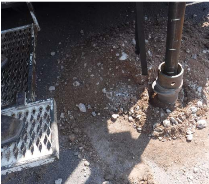
PHOTO NO. 27: General view of gravelly soils encountered in vertical boring B-2.
