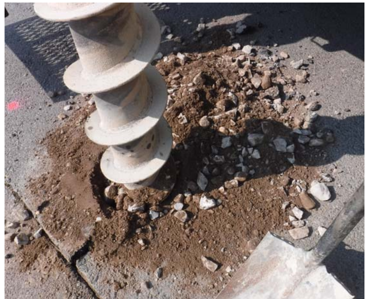
PHOTO NO. 28: General view of gravelly soils encountered in vertical boring B-1.
